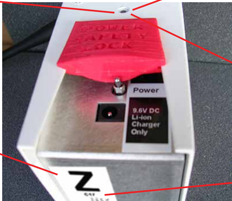
Figure 1 - T-Link2 power and external connections
